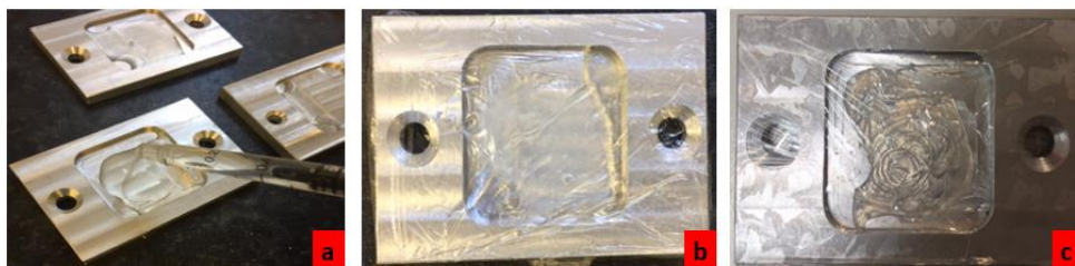
Method i) biomaterial synthesis procedure. a) synthesis of biomaterial, b) pre-setting and c) post-setting of biomaterial
