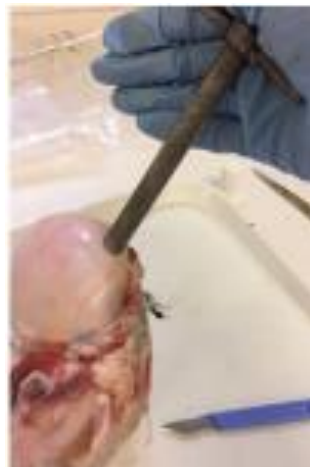
Figure 3.1: Cork boring procedure for the preparation of cartilage off-bone specimens. The cork borer is applied with force onto the surface of the cartilage humeral head, in the normal direction to the cartilage surface. This schematic is for representation purposes of the equipment rather than exact positioning of the cork-borer relative to the cartilage surface. This procedure is followed by the removal with a surgical scalpel.
