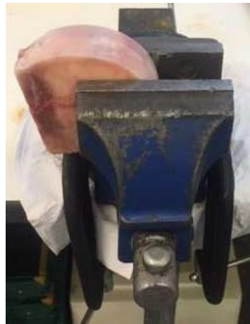
Figure 5.6: Articular cartilage specimen dissection procedure: method to obtain the central region of the humeral head for extraction of lower cartilage specimen sheets, for testing
