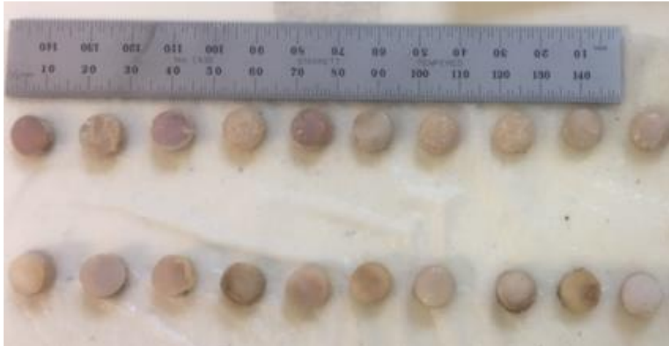
Figure 5.8: Illustration of prepared upper cartilage-on-bone specimens drilled and cut to precise dimensions for testing
