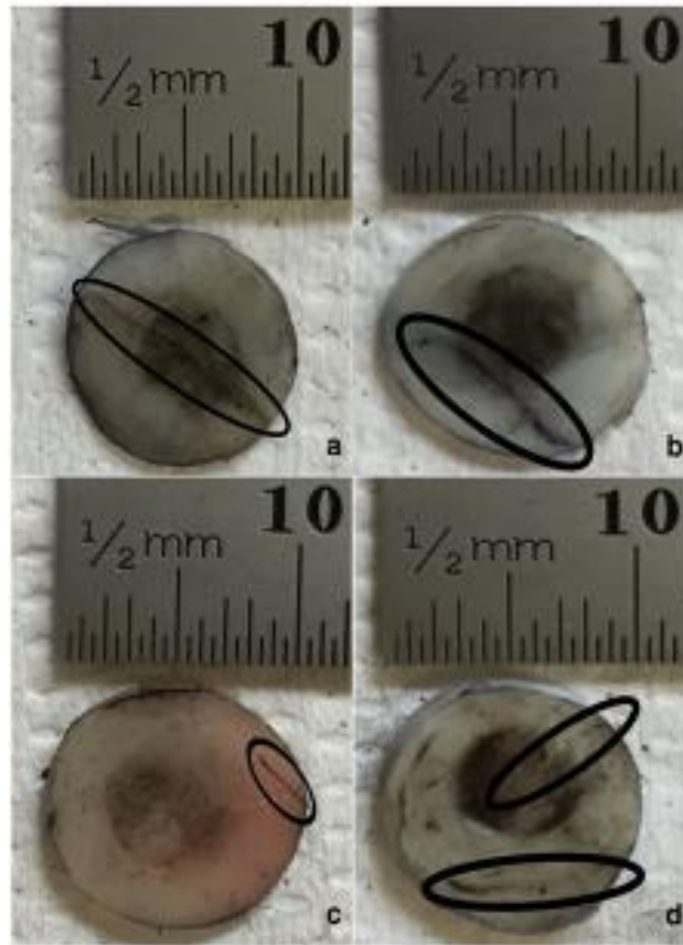
Figure 3.16: Representative images of bovine articular cartilage-off-bone samples after testing, at 50 Hz frequency of loading. Image a-d display a sample result of the highest to the lowest substrate density, identified by the densities of 0.1556, 0.3222, 0.5667 and 0.6000 g/cm 3 , respectively. Damage as cracks and indentation were identified with application of India ink. Cracks formed are highlighted with the black ellipse for clear observation, notably of single-line configurations of varying lengths. Scale bar (mm) included for quantifying results
