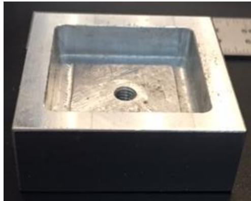
Figure 3.7: Aluminium test-rig customly designed to securely contain the substrate, above which the cartilage specimen is placed for testing.
