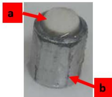
Figure 5.9: Upper specimen holder: a) the upper articular cartilage specimen core held by the upper specimen holder illustrated in part b
