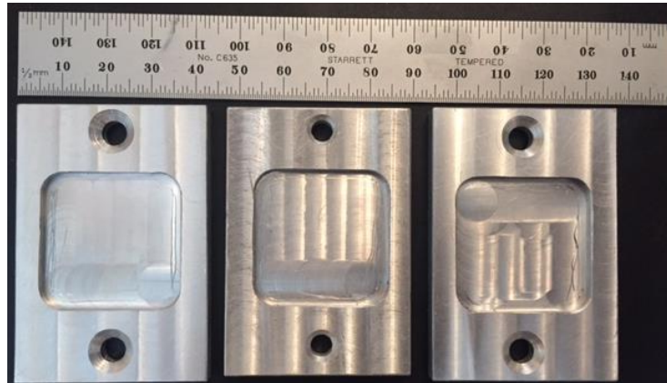
Customised aluminium test-rig manufacture to contain hydrogel for preliminary testing
