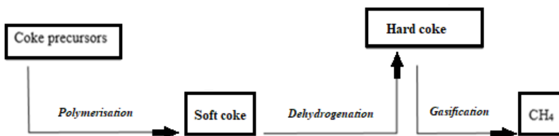
Figure 4.1 Mechanism of coke formation in upgrading reaction
