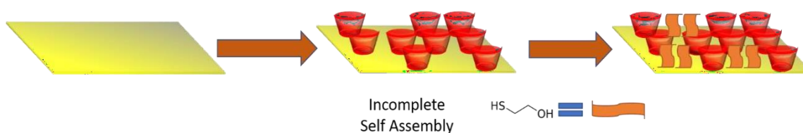
Figure 8.1.4 Diagram of the self-assembly of the spacer for the minimisation of layer imperfection. In the second step, the 2-mercaptoethanol is used in order to cover possible imperfections given by the first self-assembly of the cyclodextrin on the surface.
