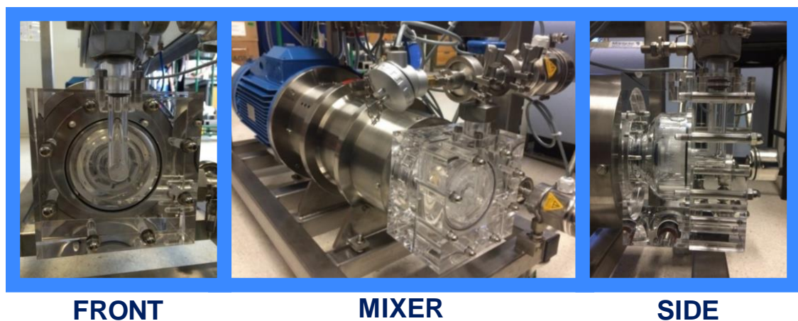
Figure 3.2: Photographs of (a) Experimental rig (b) The modified in-line Silverson 150/250 mixer
