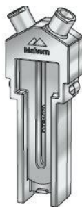
Figure 3.3 Folded capillary zeta cell used for zeta potential measurements. Adapted from Malvern Instruments Ltd. (2013).
