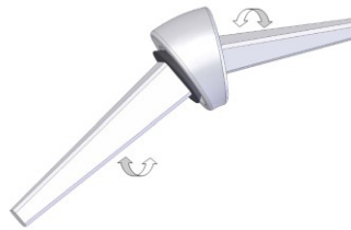
Fig 11-20 .Free rotation of the stems and heads towards the elastomer part
