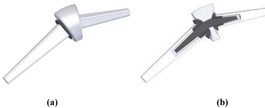
Fig 11-23. Assembly of the metacarpophalangeal final design (a) 3D view, (b) section view
