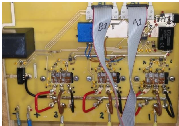
Figure 4.6: Custom-made three-phase converter power board, front side
