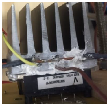
Figure 5.5: Parallel resistors inserted inside the heatsink
