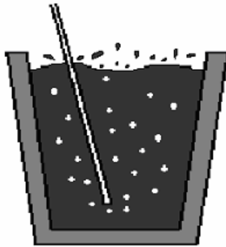
Figure 3.3: schematically shown surface turbulence during fluxing and degassing
